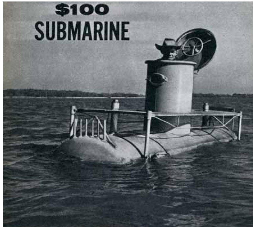
TURTLE II with Admiral Bass. Boat weighs 3,000 lbs., including 3,000-lb. cement keel.
