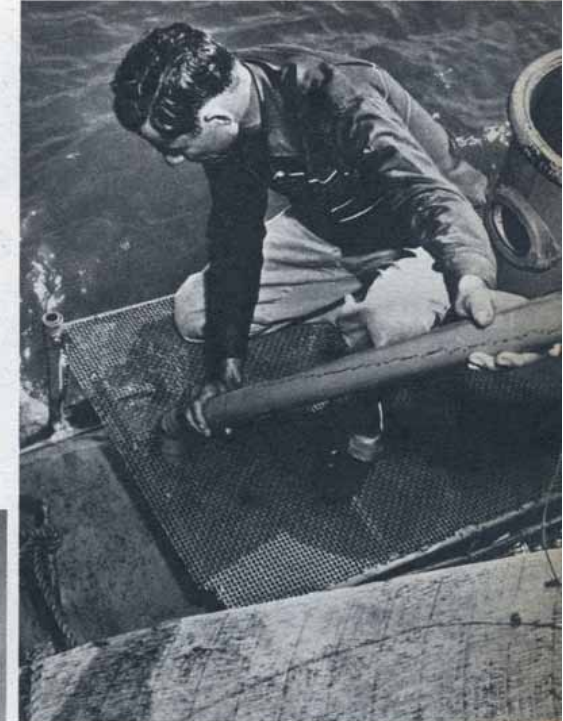
AIR is supplied by two snorkles when the Admiral wants to stay submerged. Water is kept from coming into sub in heavy seas by hollow copper float balls used in plumbing.
